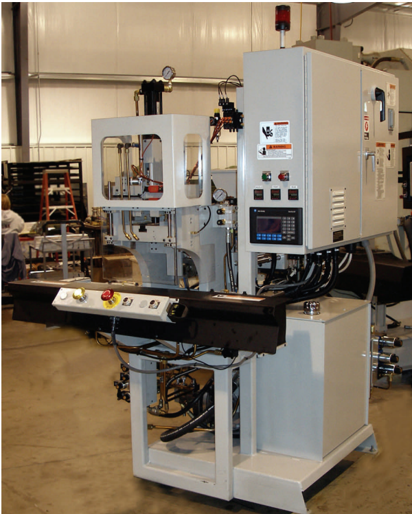
Pictured with optional Allen Bradley SLC 500 control w/ PV550 interface
